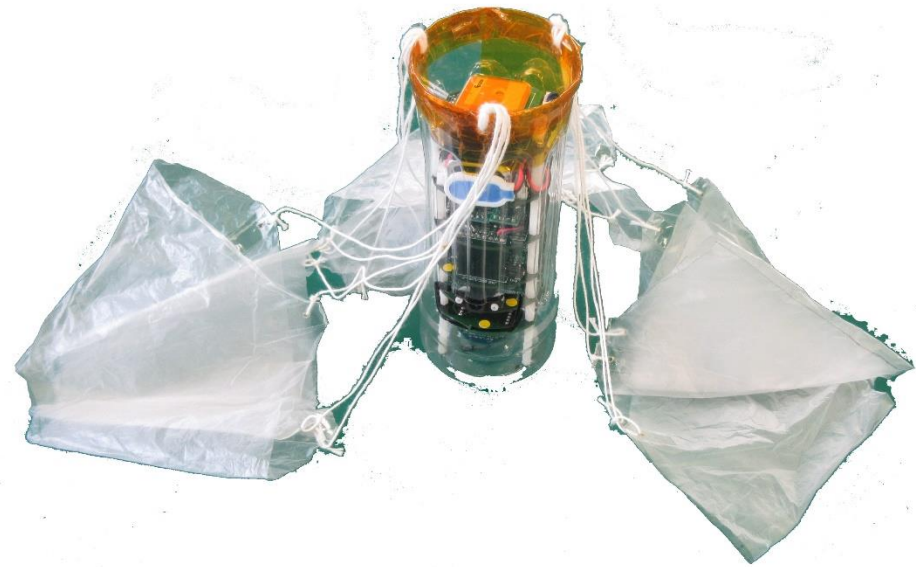
i-CanSat: Structure & Parachute
